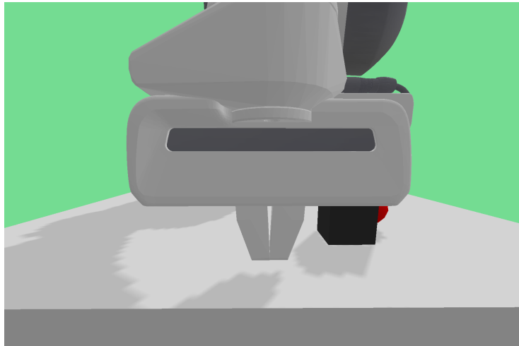
Figure 3: The collision contours of the panda robot's fingers are not parallel in simulation.
